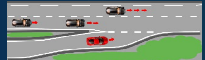
Insertion on highway of a CAV (in red) from the entry slip road
