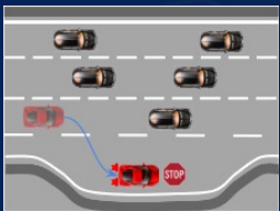
MRM performed by a CAV (in red) on highway
