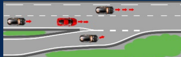
Management of the insertion of a vehicle on a highway where a CAV (in red) is approaching
